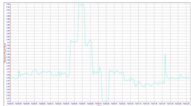
Fig. 4. Reactive power of Khourin feeder in the studied period.
